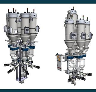
**NOSTE gravimeters** operate on a loss-in-weight principle. Gravimeter measures the material's weight to achieve and maintain a predetermined output measured in units of weight per time. The system includes line speed measurement, and you can also measure the product by width. These variables allow you to specify the weight value by length or area. It improves operator's awareness of the process and enables significant material savings.
